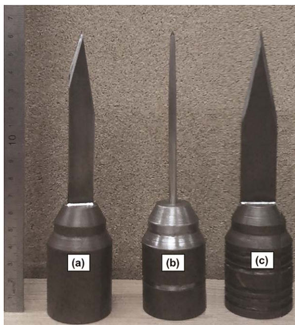
Figure 3. Weapons used: (a) P1 blade, (b) Spike, and (c) S1 blade. [Color figure can be viewed in the online issue, which is available at wileyonlinelibrary.com .]
